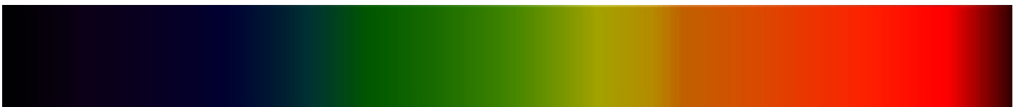
Figure 5: Incandescent emission spectrum. All visible light wavelengths are produced
